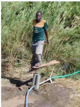
Malawi - treadle pump for irrigation
